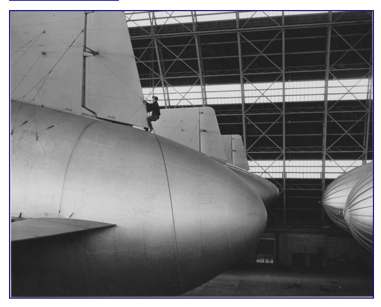
HEDRON-11 airship rigger inspecting the cables and other fittings attached to the vertical stabilizer of a ZP-11 ZNP-K type blimp inside NAS South Weymouth's LTA Hangar One sometime during the Second World War. The fins, car, and various other things connected to a blimp's rubberized fabric gasbag were mainly secured by an arrangement of steel cables. Due to the flexing of the gasbags, these cables had to be checked constantly to ensure that they were still taut and in proper alignment.
